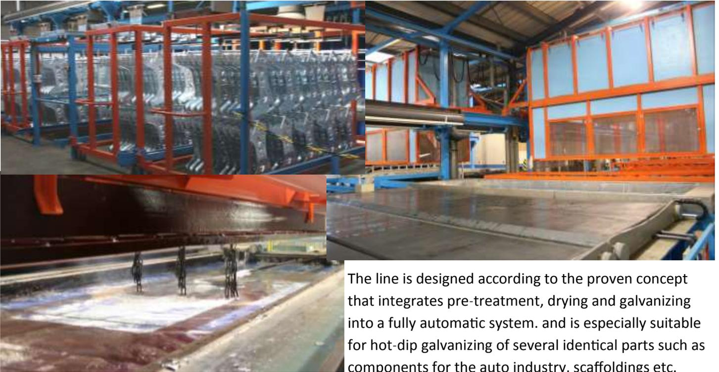
The line is designed according to the proven concept that integrates pre-treatment, drying and galvanizing into a fully automatic system. and is especially suitable for hot-dip galvanizing of several identical parts such as components for the auto industry, scaffoldings etc.
