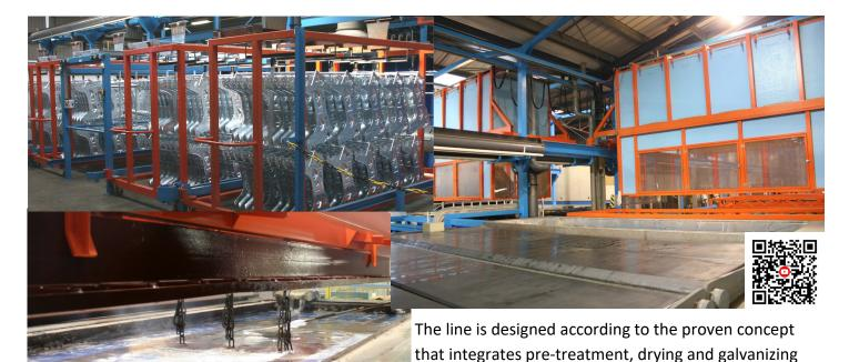
into a fully automatic system. And is especially suitable for hot-dip galvanizing of several identical parts such as components for the auto industry, scaffoldings etc.
